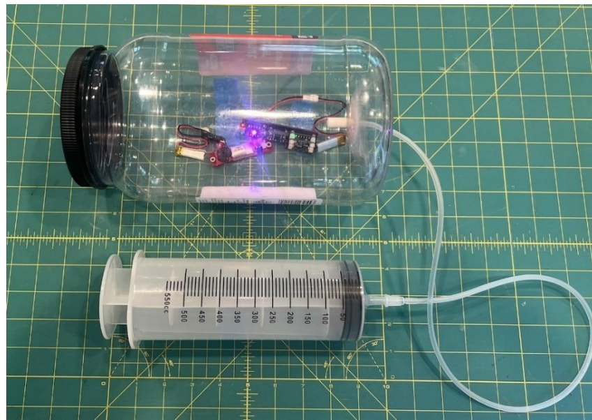
Figure 5.1-1. A simple vacuum system was developed to perform pressure/altitude accuracy tests.
